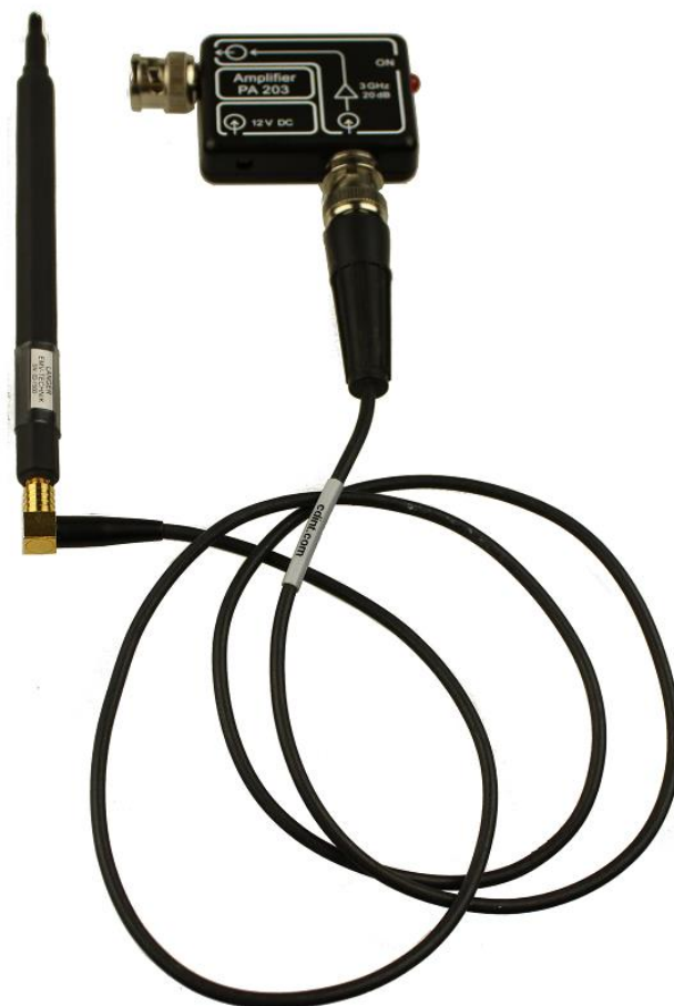
Figure 18 EM capacitor probe connected to the Amplifier
