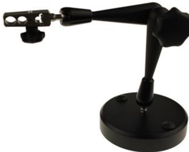
Figure 2 The complete 3D probe positioner
