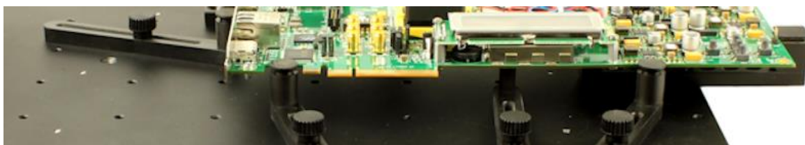
Figure 5 Close-up view on the usage of the different adjuster brackets.
