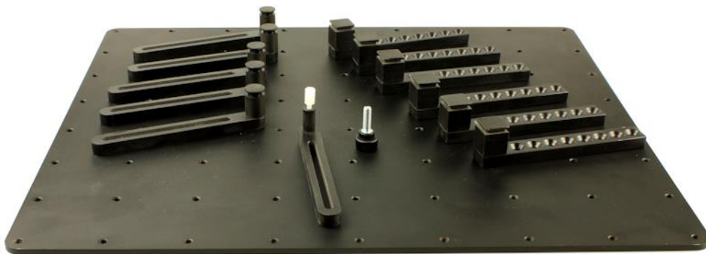
Figure 1 The fixture system based on adapter brackets on a positioning grid.
