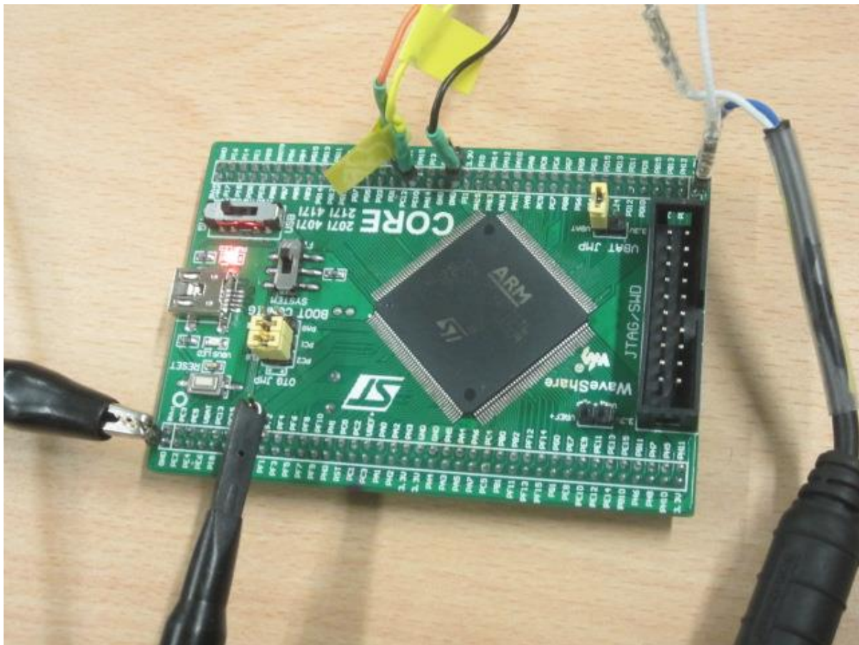
Figure 5 An example of custom wiring with an embedded target.
