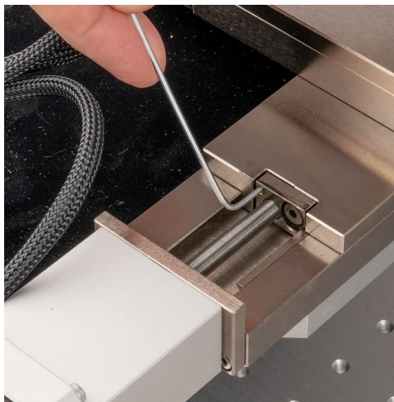
• Figure 10 Backlash adjustment screw at stage carriage.
