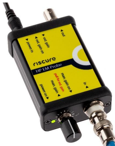
Figure 4 The “man. gain” knob is pulled out to enable external gain.
