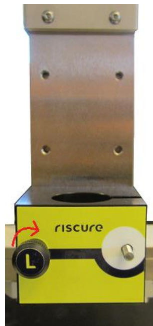
Figure 19 align the “L” screw to the drill hole on the arm and tighten it
