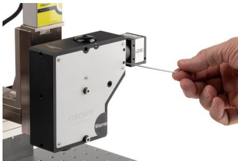
Figure 10 Loosen hex screws of C-mount flange and rotate NIR camera.
