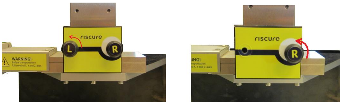
Figure 2 loosen and remove the “L” screw and “R” screw cap
