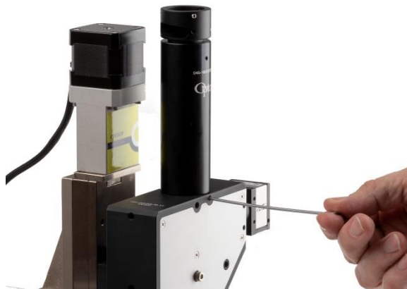
Figure 14 Mount Spot Size Reducer on top of Compact Laser Microscope body.
