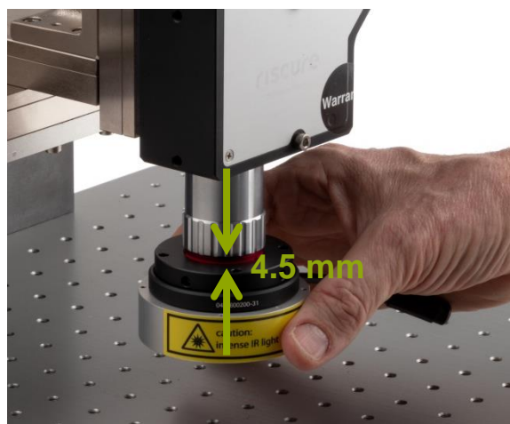
Figure 13 Mount magnetic ring and IR ring light to objective.
