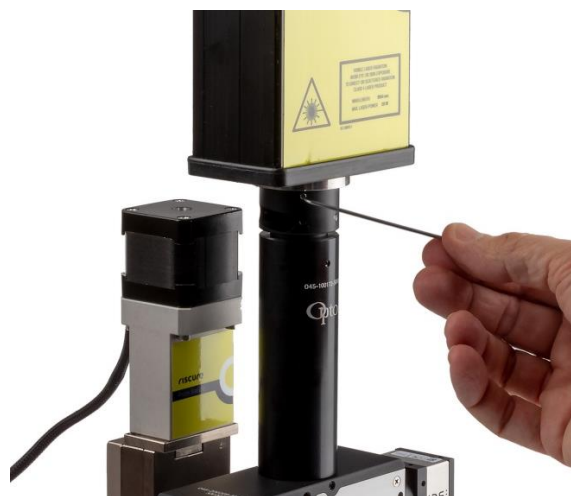
Figure 15 Mount laser on top of Spot Size Reducer.
