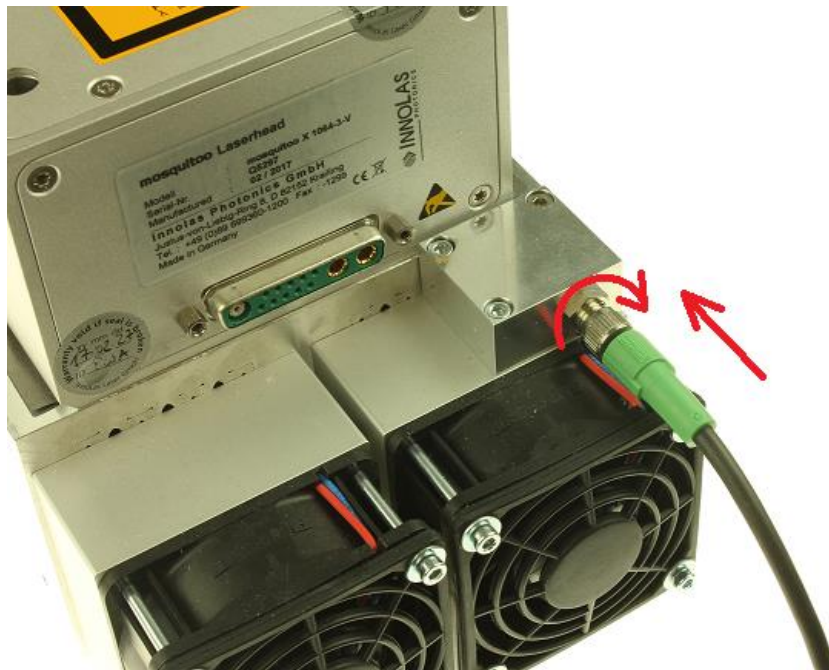
Figure 12 Connect the cooling cable to the Laser Head
