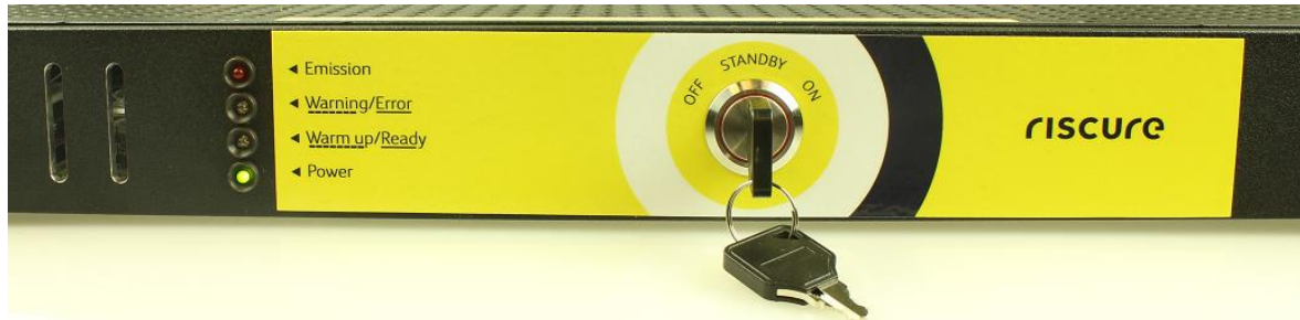
Figure 29 Key turned to "STANDBY" position, "Power" LED lighting up
