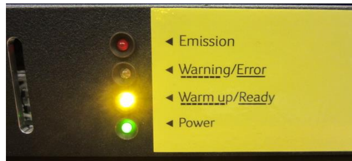
Figure 32 PSU LED state when Interlock circuits of the Riscure Safety box is Open
