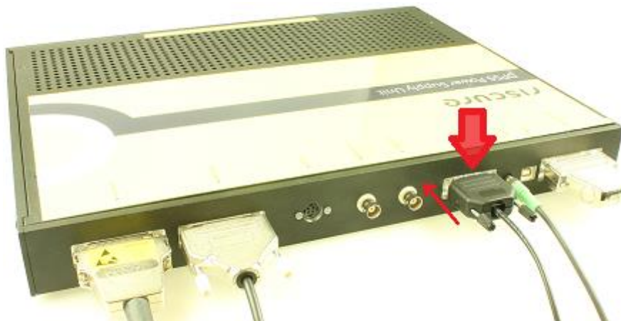
Figure 16 (with Riscure Safety box) Connect interlock cable to the PSU
