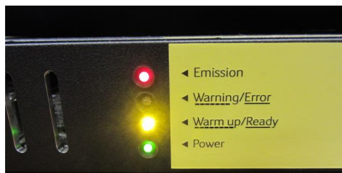
Figure 31 PSU LEDs when DPSS Laser Head is ready to fire
