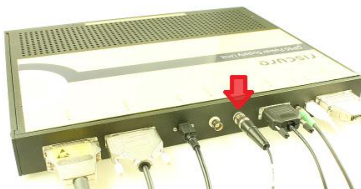
Figure 33 BNC-SMB cable that connects to either a VC Glitcher or a Spider
