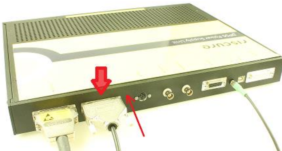
Figure 13 Connect the attenuator cable to the PSU
