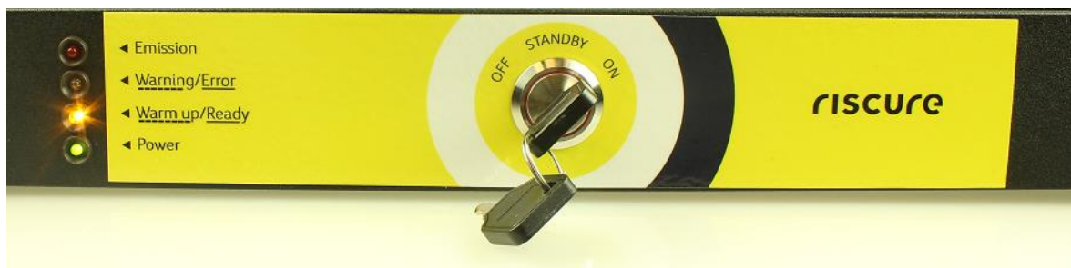
Figure 30 Key turned to "ON" position and the "Warm up/Ready" LED blinking
