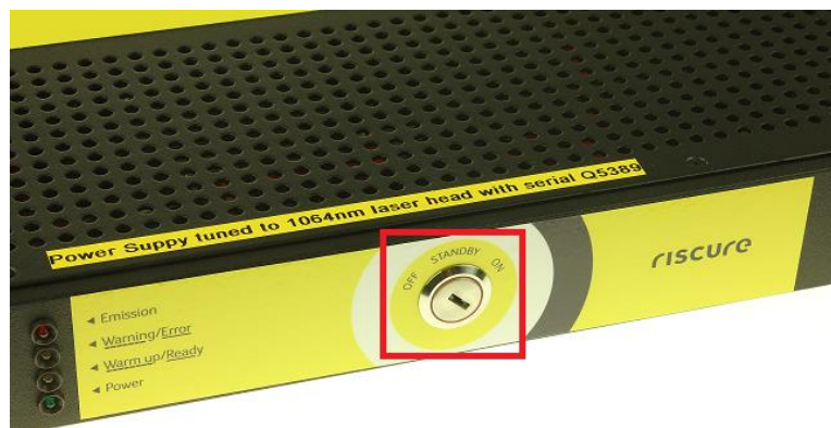
Figure 27 The key switch and available PSU states
