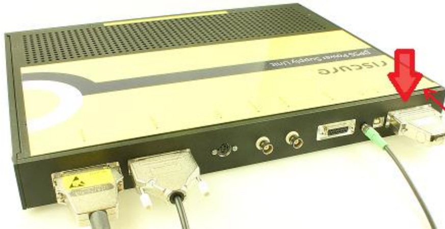
Figure 15 Connect the User Interface Dummy to the PSU
