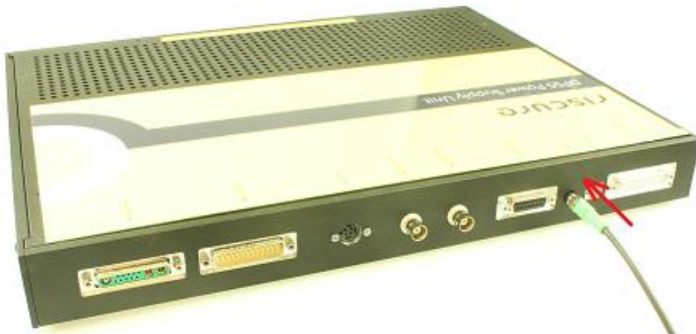
Figure 11 Cooling cable connected to the DPSS PSU
