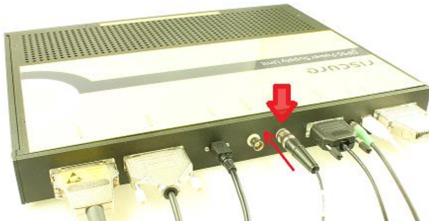
Figure 20 Connect the BNC-SMB cable to the PSU
