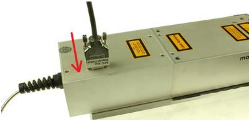
Figure 14 Connect the attenuator cable to the Laser Head
