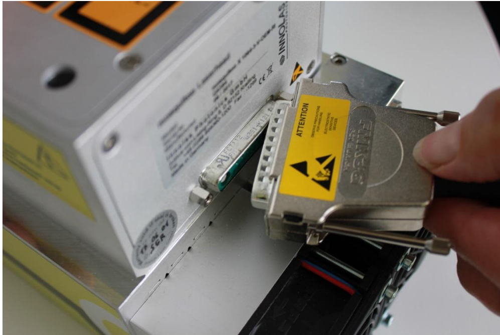
Figure 10 Be sure to connect the GND shield of the connector first
