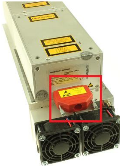
Figure 4 The Laser Head with ESD protection plug (highlighted by red rectangle)
