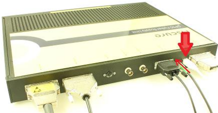
Figure 19 Connect the USB cable to the PSU
