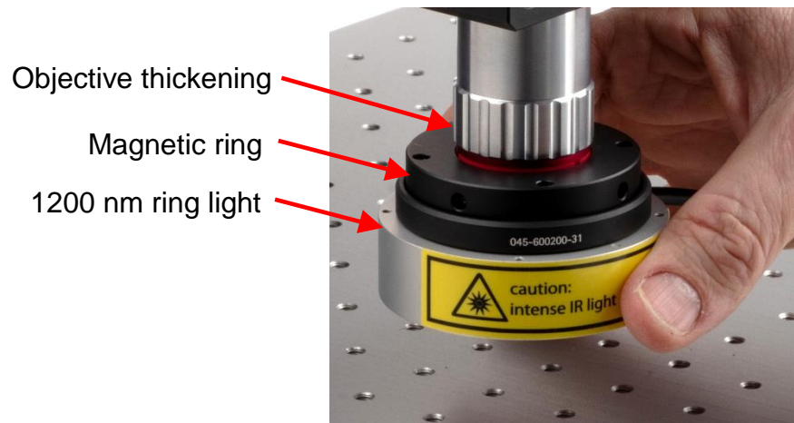
Figure 4 Mounting 1200 nm ring light to objective.
