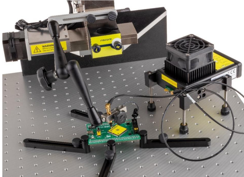
Figure 16 Glitch Needle using a XYZ-Stage
