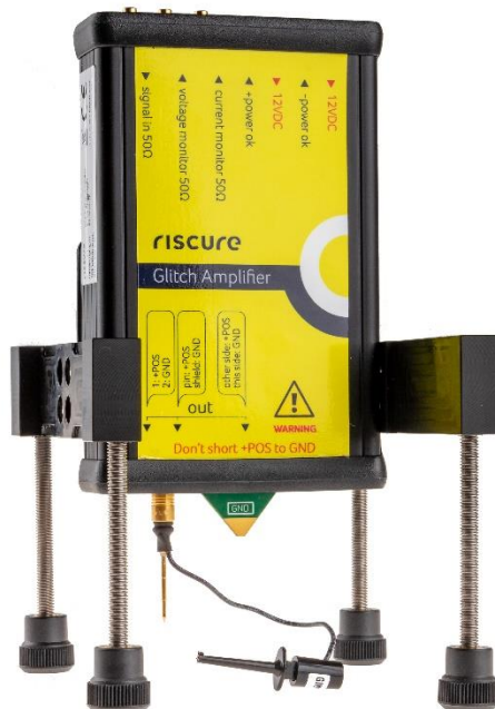
Figure 17 Glitch Needle Directly mounted on Glitch Amplifier
