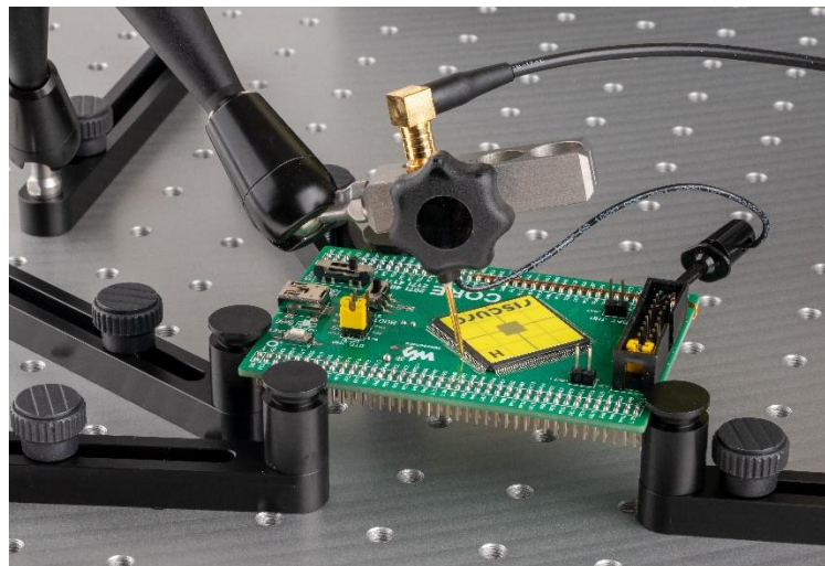
Figure 11 Glitch Needle setup on a Piñata target using a Riscure XYZ Stage and 3D positioner.
