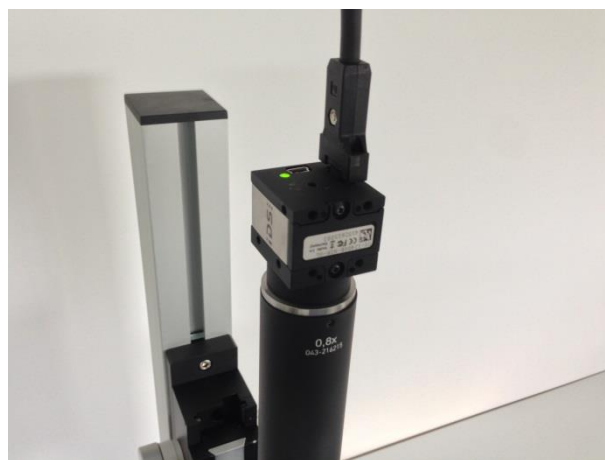
Mounting of IDS UI-1240E-NIR-GL camera on camera tube of microscope
