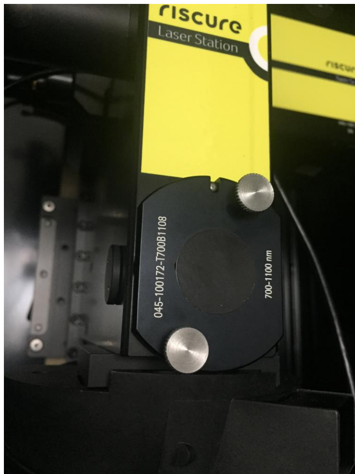
LS-2 body with Beam splitter mounted
