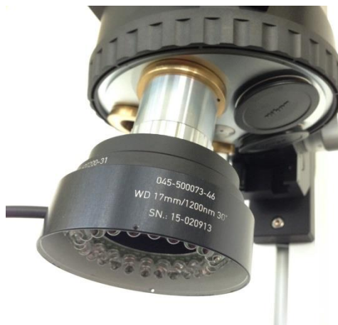
Attaching 17 mm WD IR ring light to magnet ring on 5x objective
