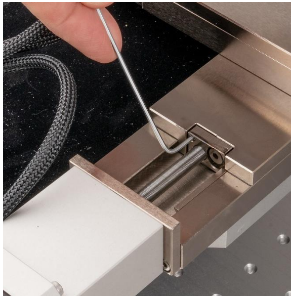
• Figure 10 Backlash adjustment screw at stage carriage.
