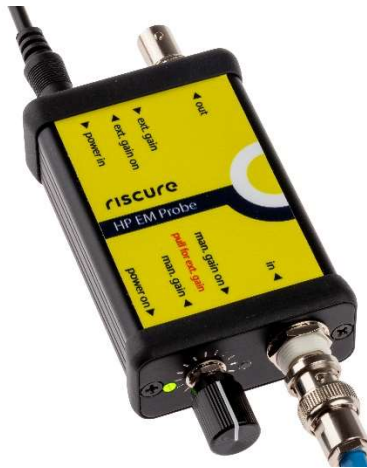
Figure 7 The “man. gain” knob is pulled out to enable external gain.
